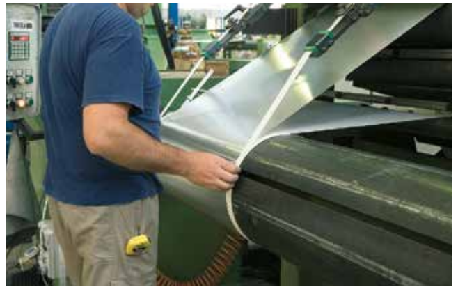
LV winding system
